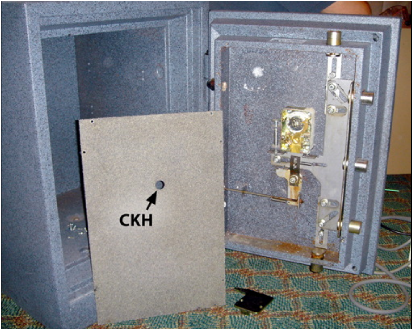
Back side of door with back panel removed. Arrow points to change key hole (CKH) in the panel. Hmm, so if there is a CKH in the panel, why did I say that scoping the CKH was not easy? The answer in a moment.
