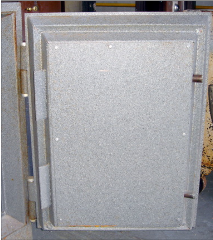
◀ Back side of door with back panel attached. Notice there is no CKH. This makes sense, since there is no changing index on the dial ring either.
